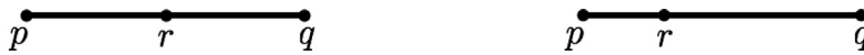
Fig. 4. The new node of the edge pq (left–right): no singular vertices (midpoint); p is a singular point ( |pr| = \kappa_p|pq| , \kappa_p < 0.5 ).
